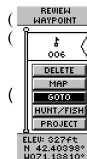
The compass page will appear with distance and a direction to find what has been marked. Remember, the arrow only works while you are moving and once you are within 20 feet you should be on top of what was marked.
